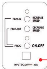
Through two buttons on the control panel it is possible to increase or decrease the rotation speed of the units. The control panel allows to set also the label rewinding face-in or face-out option. (just on rewinder units)
