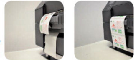
The printed media or liner will pass underneath the printer.
